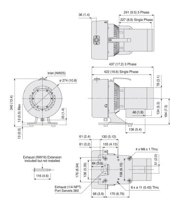
The TriScroll series is a range of two-stage dry scroll pumps that have high pumping speeds and low base pressure. TriScroll pumps eliminate the frequent maintenance requirements of oil-sealed rotary vane pumps, simplifying regulatory and environmental compliance, and eliminating oil disposal costs. The unique, patented TriScroll pump offers proven reliability and durability, delivering consistent performance and superior cost of ownership.
